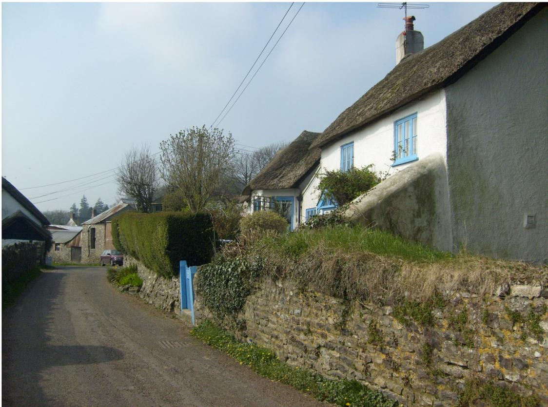
construction is relatively well coursed and bedded in a course lime mortar. Render is roughcast on the whole with later work on some properties in a
